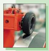
Single position vertical noise tester designed to operate at a very low noise level to provide optimum conditions for the measurement of tire generated noise.
