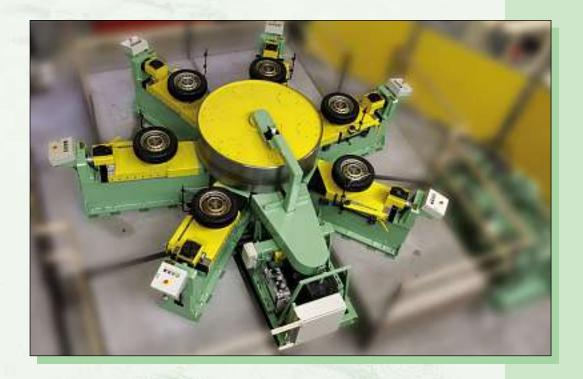
Horizontally aligned road wheel, designed for tire endurance testing with up to six tires to be tested simultaneously.
