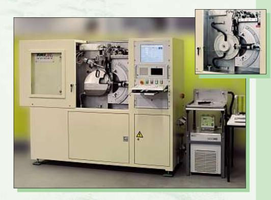
Laboratory tester for measurement of skid, traction, rolling resistance and wear resistance of (tread) compounds with a special disc simulation road conditions.
