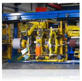
Through our decentralised design and the distribution of various modules into different control cabinets and separate pneumatics, any faults can be located immediately, start-up is much faster and the machine configuration remains flexible. We believe in development, which is why our machines have a modular design. The development, design, detailing and drafting of the tire building machines is conducted using state-of-the-art 3D CAD calculations use the Finite Element Method.
