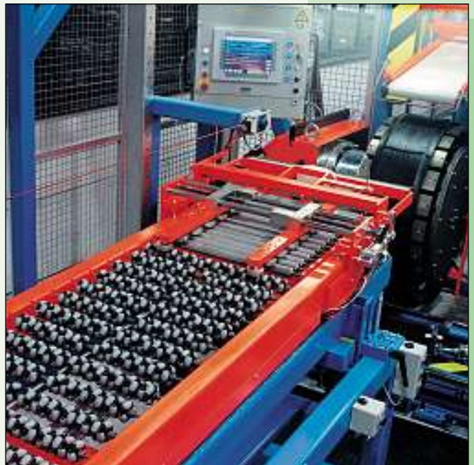
Multi size belt and tread application drum
