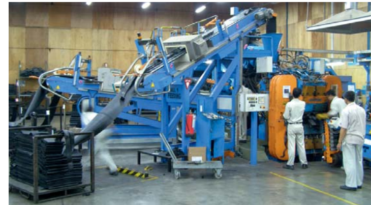
TROESTER CoEx 4/C with slab feeders Cushion calender TROESTER CoEx 3/H Rotating cross cutter as part of a wind-up system Cassette wind-up station
