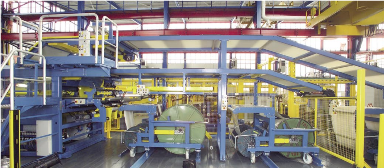
4 Automatic ply server for assembled innerliner (PA) and one or two carcass plies (BP)
