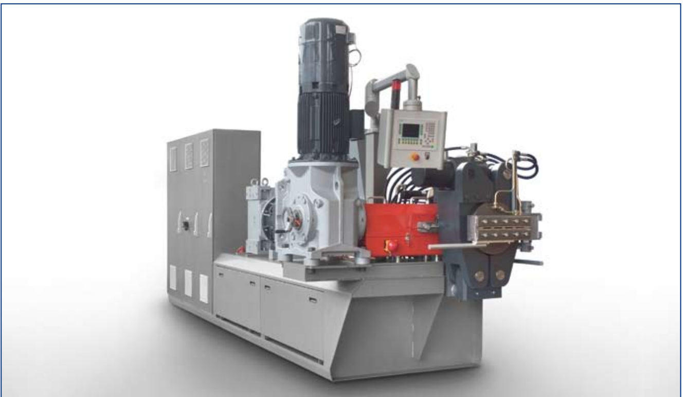
Gear pump utilized to increase pressure in a 150 mm strainer extruder, capacity approx. 1,600 kg/h
