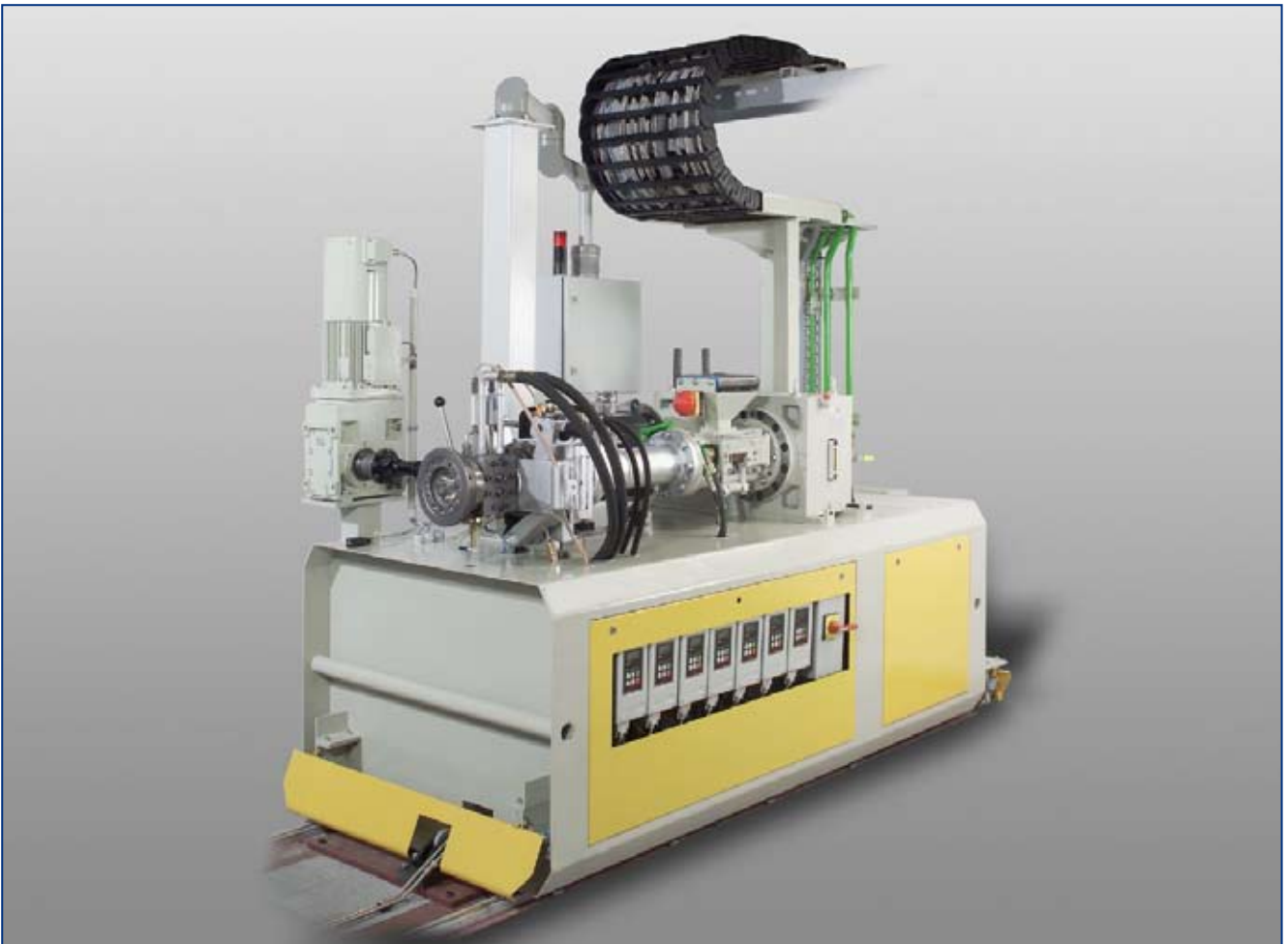
Gear pump employed to increase pressure in cross head
