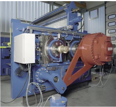
Two 550 x 1500 mm heavy-duty mixing mills with individual roll drive for variable roll speeds, hydraulic roll nip adjustment and stockblender.
