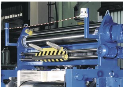
Stockblender (optional), for rapid compound cooling and increased homogeneity.
