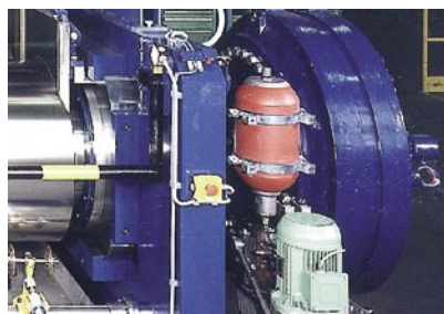
Hydraulic roll nip adjustment with pressure accumulator for rapid roll nip opening following the operation of the emergency stop.
