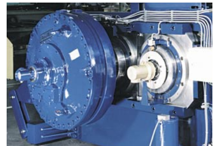
Individual roll drive through hydraulic motors and power pack.
