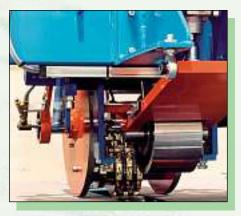
• Automatic hot sampler unit on inlet conveyor, automatically cutting out sample discs from the compound slab and automatic printing of batch number on sample.
