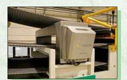
· Metal detector on outlet conveyor
