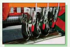
• Basic slitter system with splicer roll in the background
