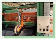
· Impression batch printer on inlet conveyor
