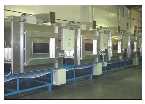
The above picture shows a Continuous Microwave oven using two TMC75 applicators of approximately 72" long x 66" wide and 52" high terminated on each end with vestibules.
