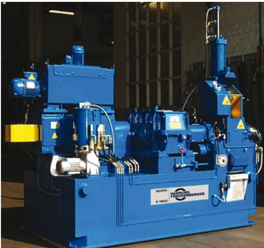
GK 1,5 E Laboratory internal mixer with pneumatic ram
