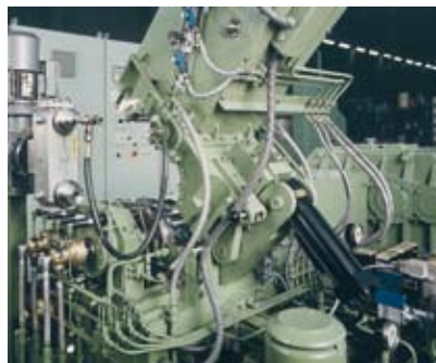
Hydraulic tilt mechanism for the top half of the mixing chamber (Typical example)
