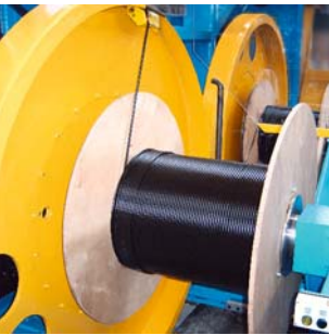
Dual Capstan DAF in a core insulation line
