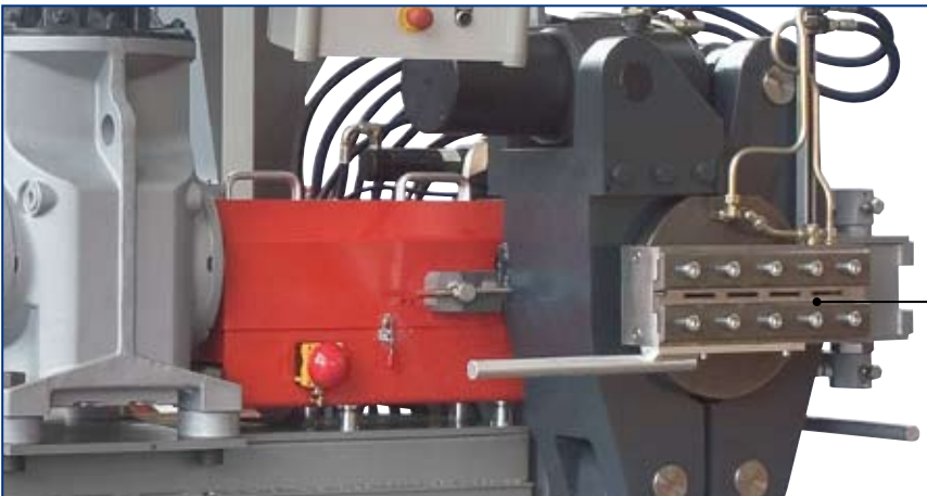
Die holder including die, and hydraulic clamp ring
