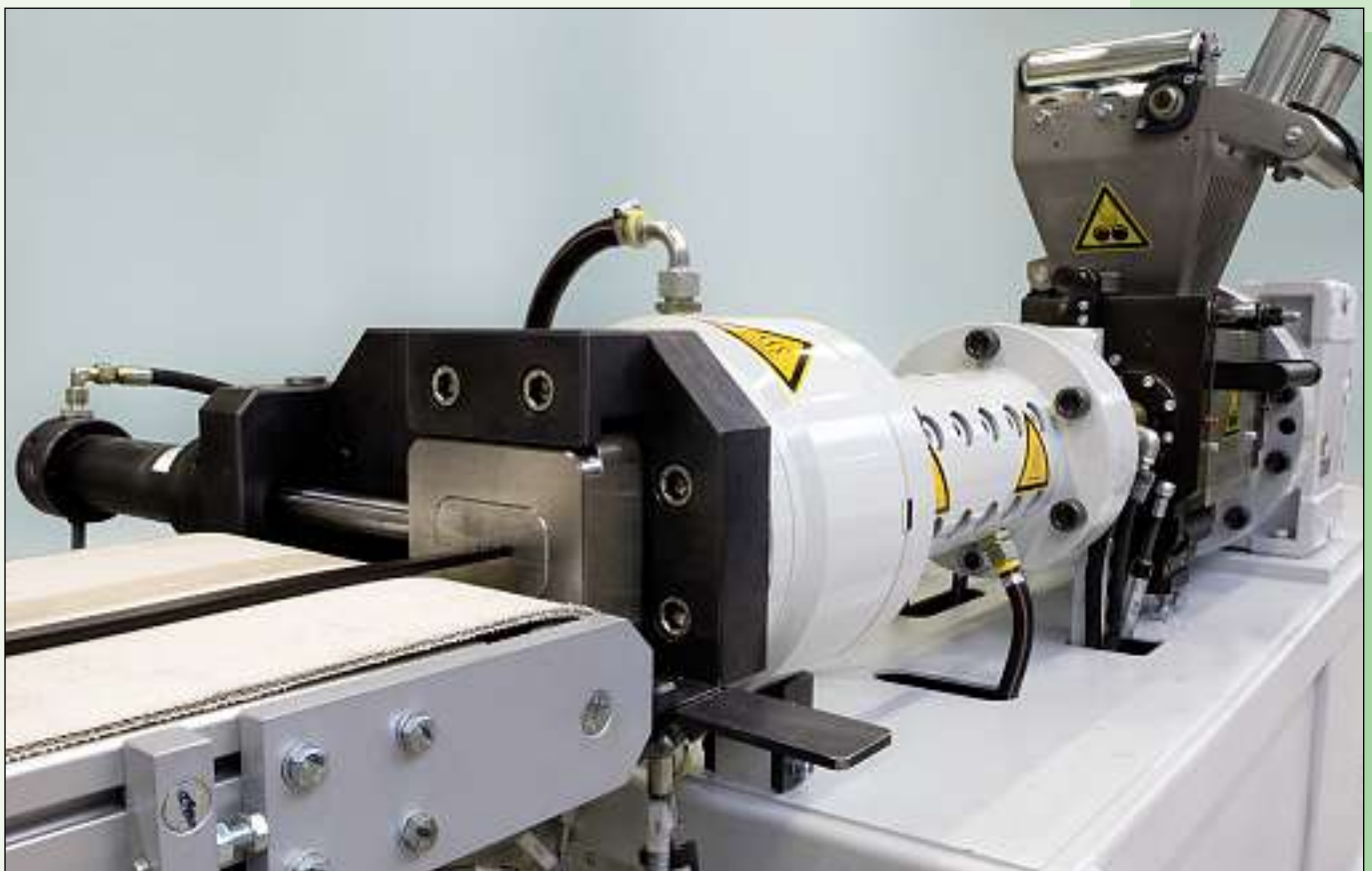
VMI-AZ Pin-barrel Extruder with quick die change head
